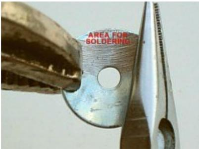
Using 2 pliers, bend the washer so that it will fit inside the PVC tube. Keep the area for soldering as depicted!
