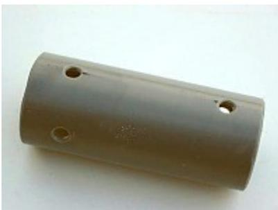
Drill all 4 holes with 5mm and remove sharp edges with a trimmer, especially for the coax holes
