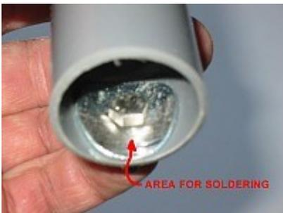
Now insert the 4 big washers in the tube ends, keep the area for soldering on the outer side, and insert the M5 bolts.
