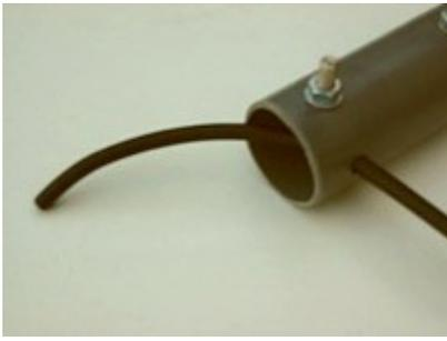
Take 93 **(153) (67)** cm of RG-58C/U coax for each coil. Insert approx 10 cm in the hole for the 'start'. RG-58C/U will just pass in a 5mm hole.
