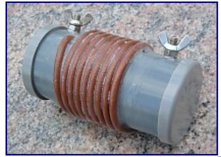
Melted and short-circuited 20m trap... power 800w SSB.
