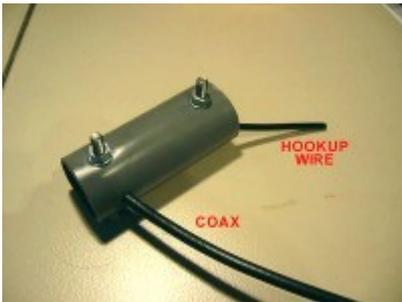
Now gently retract the coax in the tube, while inserting the hookup wire till it comes out of the tube on the other side, and the coax cannot be pulled out any more (nylon fastener)
