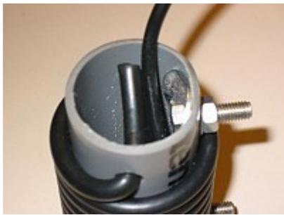
Use the short remaining end of coax to pull it as much as possible inside the tube and have windings sitting tight. Then cut off the coax so you have 20mm left inside the tube.
