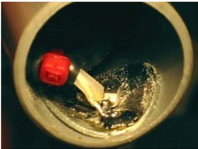
Now solder (a 60w iron should be OK) the coax center on the big washer. Make sure you have a good bond, but do not overheat as the coax / PVC will melt...
