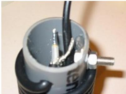
Using a cutter knife delicately around outer jacket, remove insulation on about 15mm and prepare coax ends like shown.
