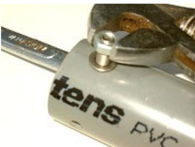
Now put the small washer and M5 nut on the bolts and tighten very well with appropriate tools.
