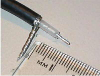
Remove insulation on 15mm of the end passed through pipe and prepare tail like shown
